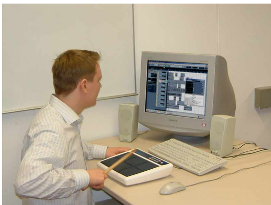
Figure 1: The setup of the BeatBank system consisting of a MIDI e-drum and the computer hosting the plug-in.
