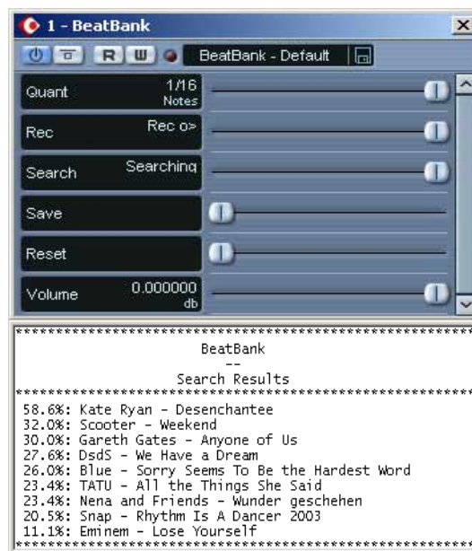
Figure 2: Interface window of the BeatBank plug-in (version 1.0). All necessary parameter settings are made in the upper part. The lower part presents the search results with the similarity values at the left side.
