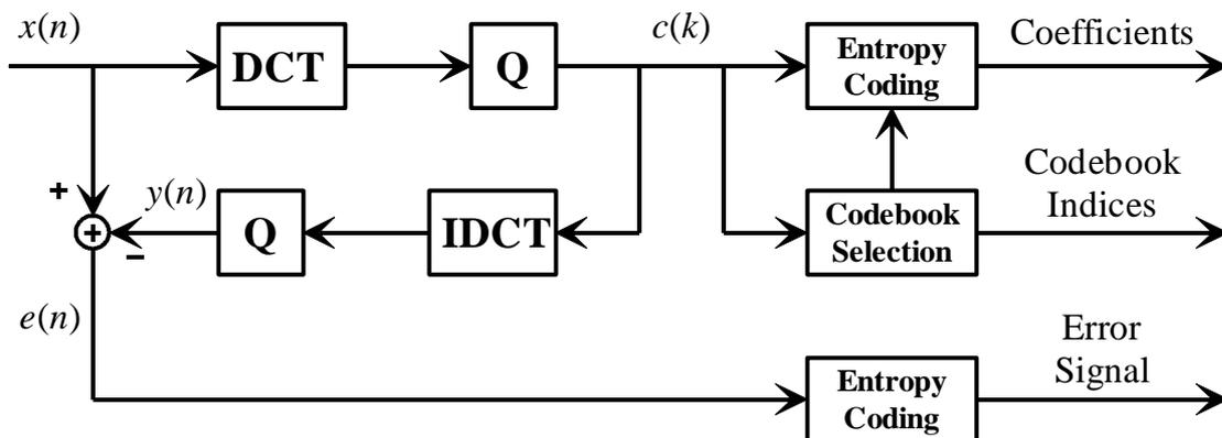
**Fig. 4:** Simplified block diagram of the implemented lossless transform coding system. Q: Quantization with step size  $\Delta = 1 / \alpha$ .
