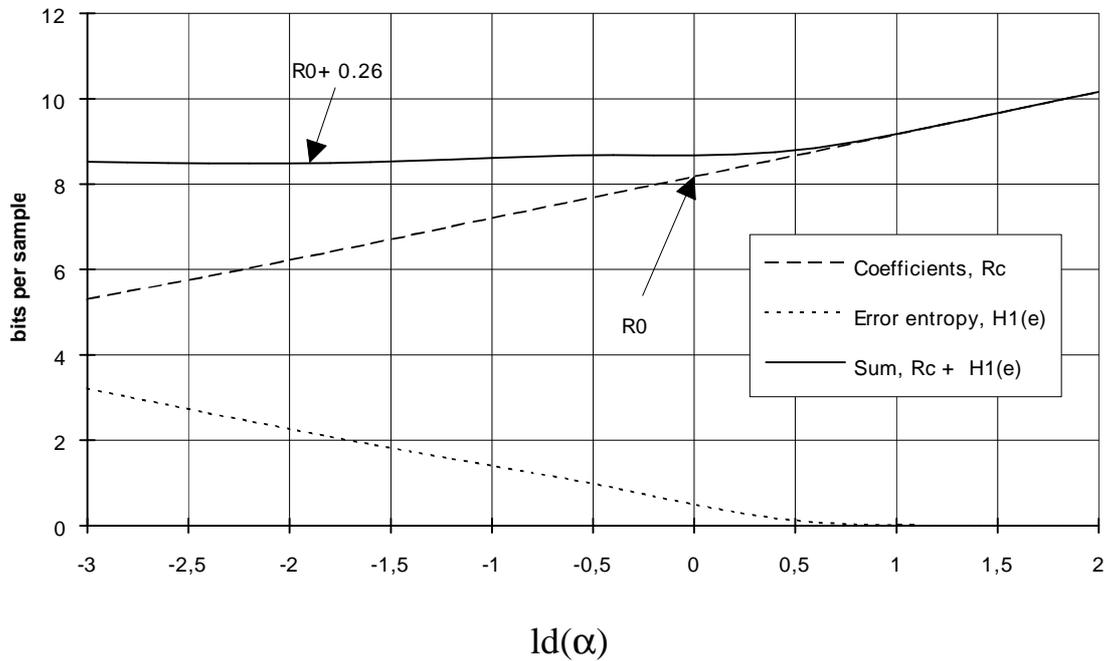
**Fig. 3:** Bit rates depending on the scalefactor. The values have been measured for a piece of pop music.
