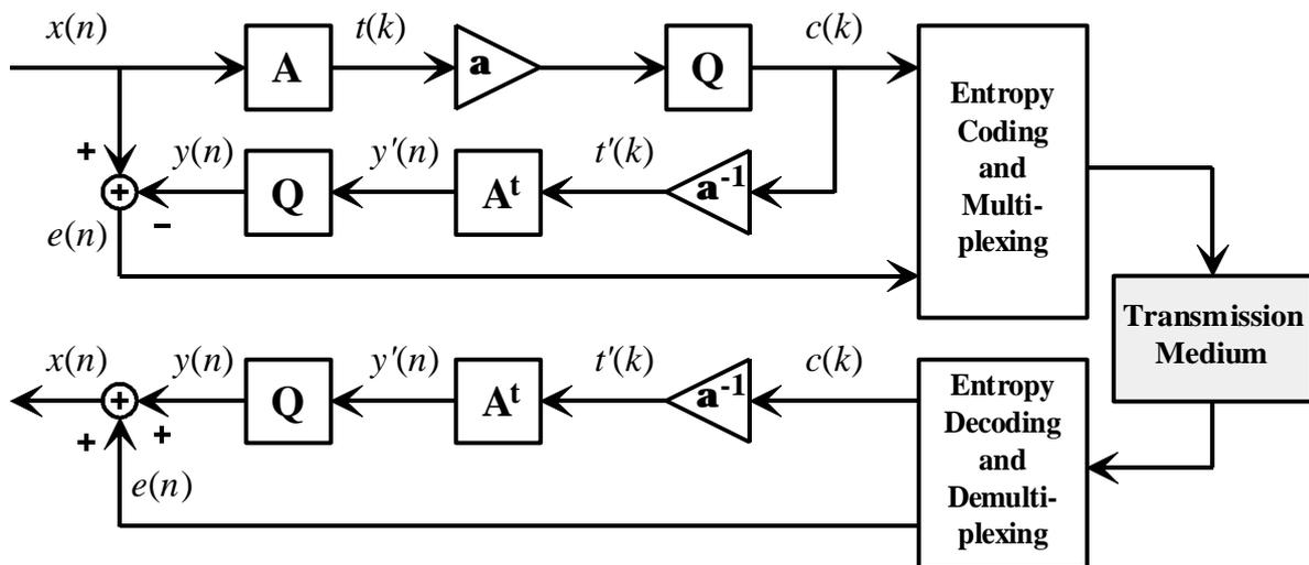
**Fig. 2:** Block diagram of a lossless transform coding system. Q: Quantization with step size  $\Delta = 1$ .
