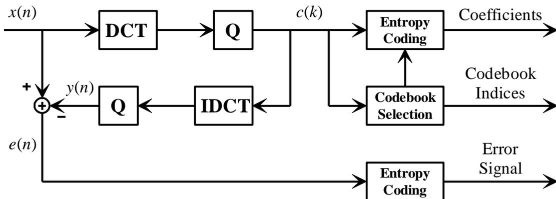
**Fig. 4:** Simplified block diagram of the implemented lossless transform coding system. Q: Quantization with step size  $\Delta = 1 / \alpha$ .
