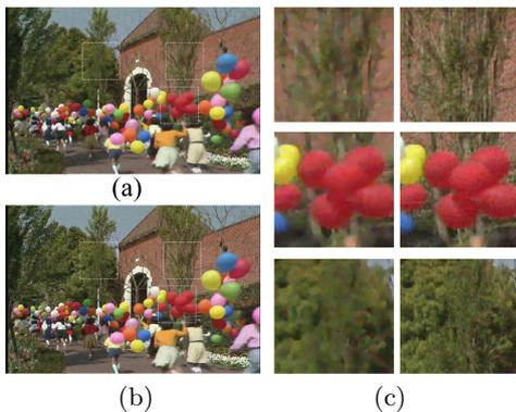
**Fig. 4** (a) Perona and Malik color diffusion for 10% Gaussian noise image, PSNR=26.199dB (b) Proposed method for 10% Gaussian noise image, PSNR=33.518dB (c) details with over-diffusion on weak edges (left: 4a, right: 4b).
