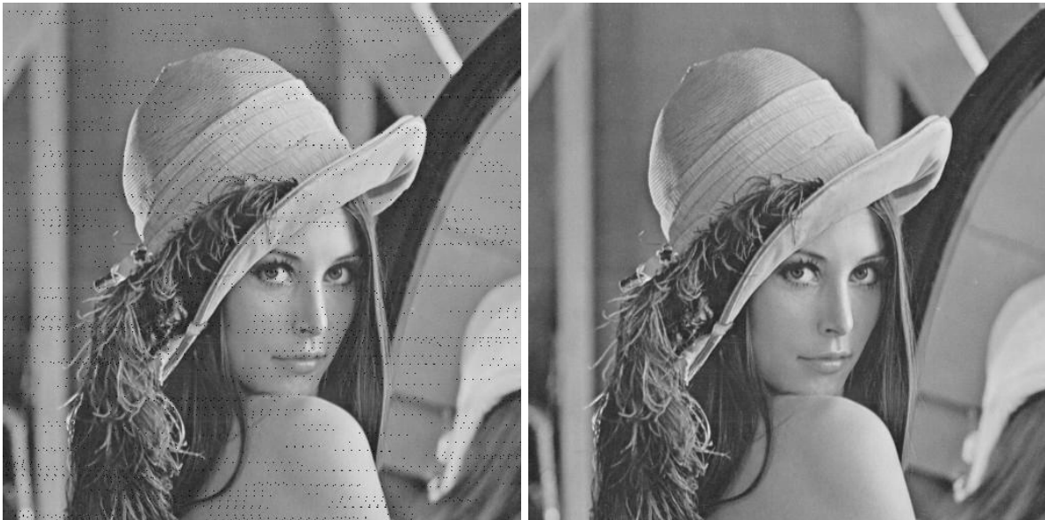
Figure 7. Result for the Identity transform, without (left) and with (right) the global optimal estimator ( H = 7.26 \text{ bpp} ).
