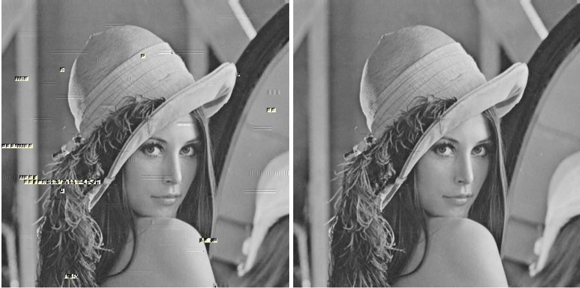
Figure 10. Result for the CCT transform ( \varepsilon = 0.08 ), without (left) and with (right) the global optimal estimator ( H = 5.81 \text{ bpp} ).
