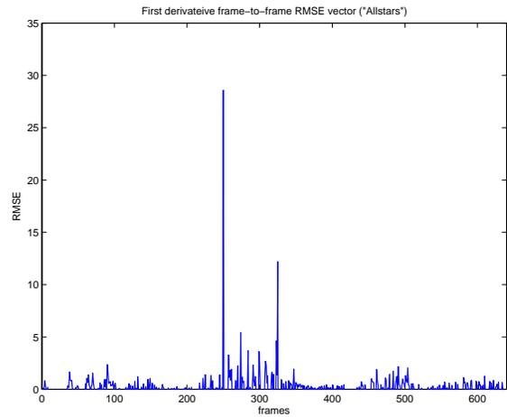
**Fig. 3.** First numerical derivative of the RMSE in Fig. 2
