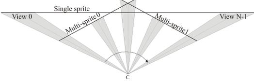
**Fig. 3.** Partition of a sequence into multi-sprites for panning camera with constant focal length
