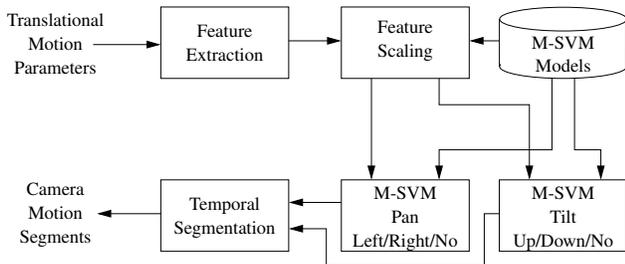
**Fig. 1.** Camera motion characterization for pan left, pan right, no pan, tilt up, tilt down, and no tilt
