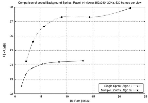
Fig. 9. Rate-distortion curve of the considered sprite generation methods, “Race1”, 4 views, 530 frames per view
