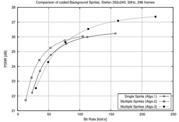
Fig. 8. Rate-distortion curve of the considered sprite generation methods, “Stefan”, 298 frames
