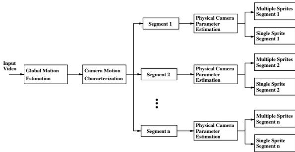
**Fig. 4.** Multiple Sprite Generation using CMC
