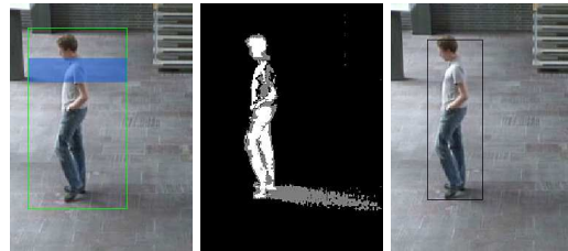
Figure 2: Left: alignment of the bounding box with the sector overlapping with the upper body part (blue). Middle: foreground mask with detected shadow regions (gray). Right: aligned bounding box.
