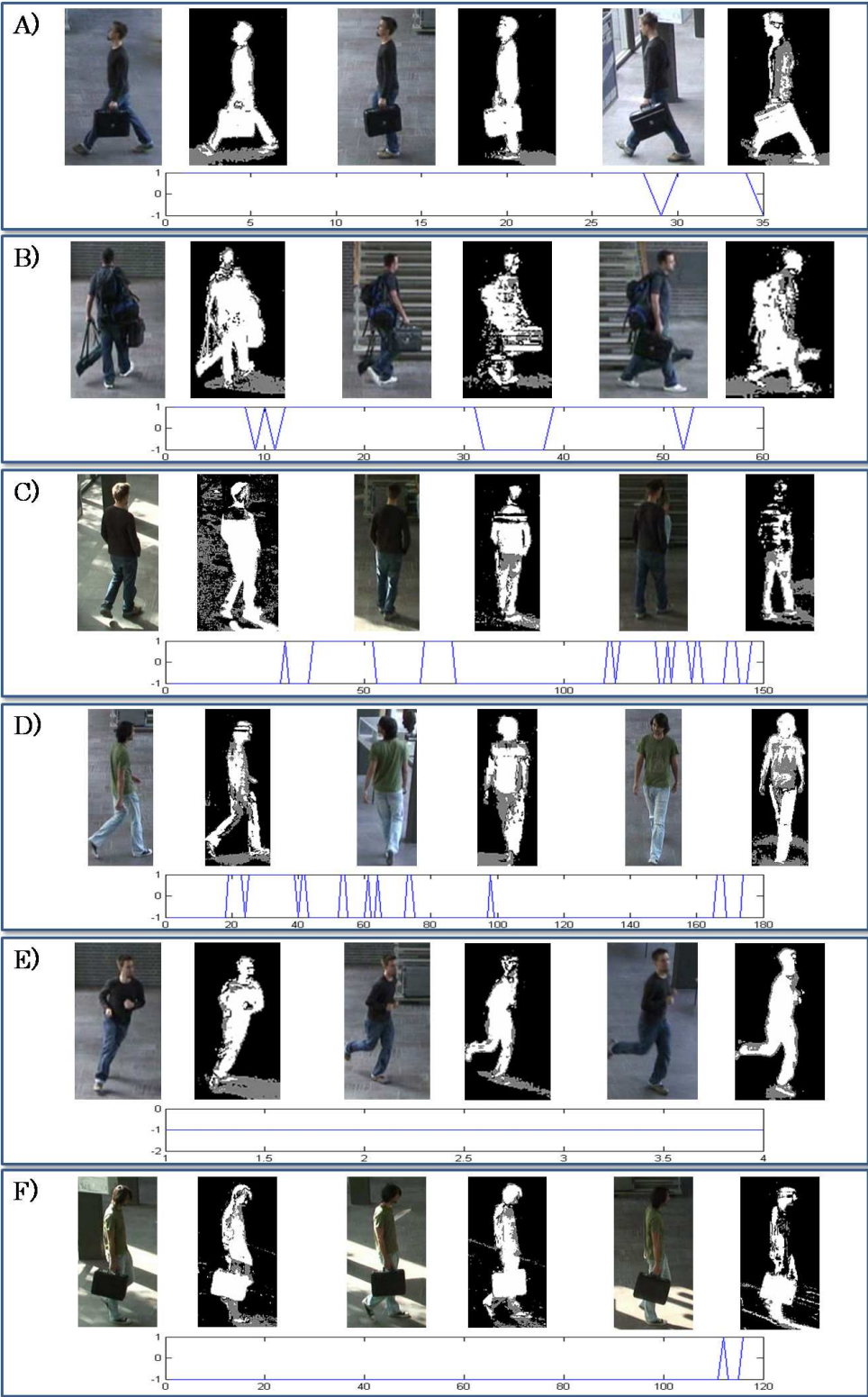
Figure 6: Width series and their corresponding classification functions. A-E: correctly classified and F: wrongly classified.
