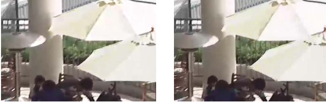
Fig. 5. A segment from frame 160 of the BQTerrace sequence, left : H.264/AVC at 3.596MBit/s (31.14 dB), right : H.264/AVC+TTF at 3.203MBit/s (31.32 dB). Especially in the fence more detail is present in the TTF filtered version.
