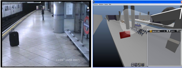
Figure 5. Model-based representation of the lost-baggage-analysis: The video stream is analyzed and new static regions are detected and represented in the 3D-model and in a system event list which contains the detection results for all cameras in the network.
