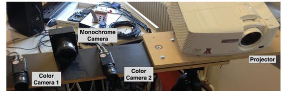
Fig. 3. Hardware configuration of the 3D-scanning unit.
