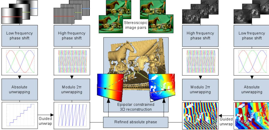
Fig. 2. Schematic diagram of the PMT algorithm [3].
