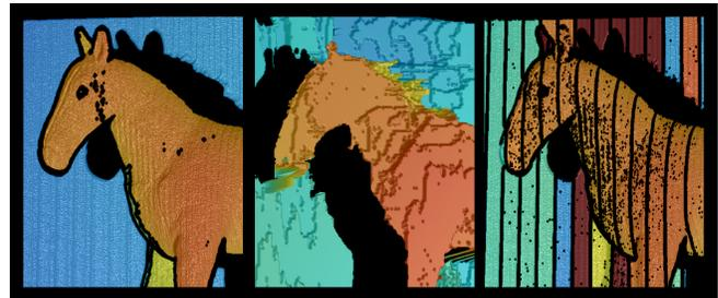
Fig. 1. 3D-reconstructions. From left to right: PMT, PCF, SPU.
