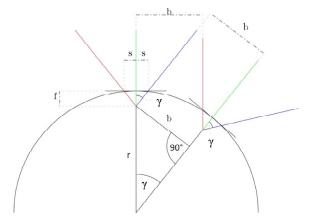
Figure 1: Schematic concept of concentric mosaics and geometric relationships for the calculation of column distances s.
