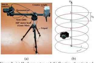
Figure 2: (a) Hardware setup and (b) Creation of vertical subaperture panorama images (r = 36.8cm and  $\Delta_H = 2.3cm$ ).
