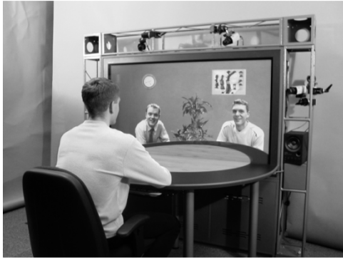
Fig. 12. Immersive virtual environment video conference setup (FhG HHI, Berlin, Germany). Persons from different remote locations are arranged around a virtual table. Each participant can be compressed as arbitrarily shaped video object using the MPEG-4 object-based coding modes.
