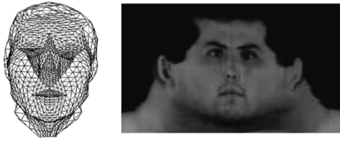
Fig. 15. 3-D model and SPRITE image of a person used for model-based coding (Source: P. Eisert, FhG HHI, Berlin).
