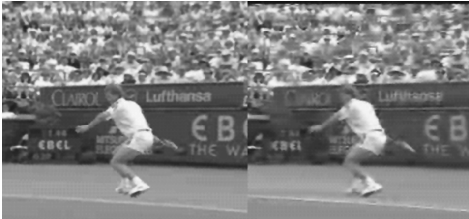
Fig. 14. Comparison of MPEG-4 SPRITE coded TV video (left) versus standard MPEG-4 block-based MC/DCT coding at 1 Mb/s (right).
