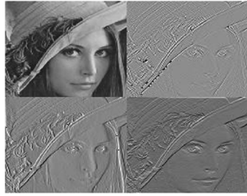
Fig. 3. Predictive coding of test image “Lenna.” Top left: original image. Top right: 2-D prediction. Bottom left: 1-D prediction, B = C = 0 . Bottom right: 1-D prediction, A = C = 0 .
