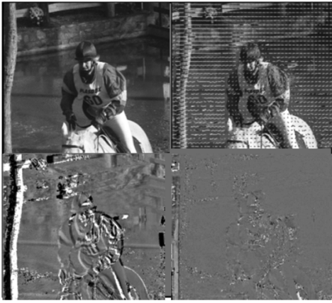
Fig. 9. Efficiency of MPEG/ITU-type video coding using block-based motion prediction. Top left: frame to be coded. Top right: estimated motion vectors \underline{x} for each 16 \times 16 block. Bottom right: motion compensated prediction error image. Bottom left: prediction error using simple frame difference (all motion vectors are assumed zero).
