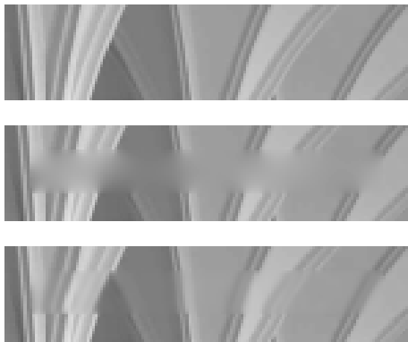
Fig. 6: Results of error concealment: original block (top), mono concealment (center), 3D-BS algorithm (bottom)
