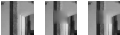
Fig. 7: Results of error concealment: original block (left), mono concealment (center), 3D-BS algorithm (right)
