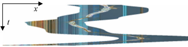
Fig. 3 Image of mosaic pixel candidates over time t for the line y = 90 of sequence "Stefan" (see the foreground object)
