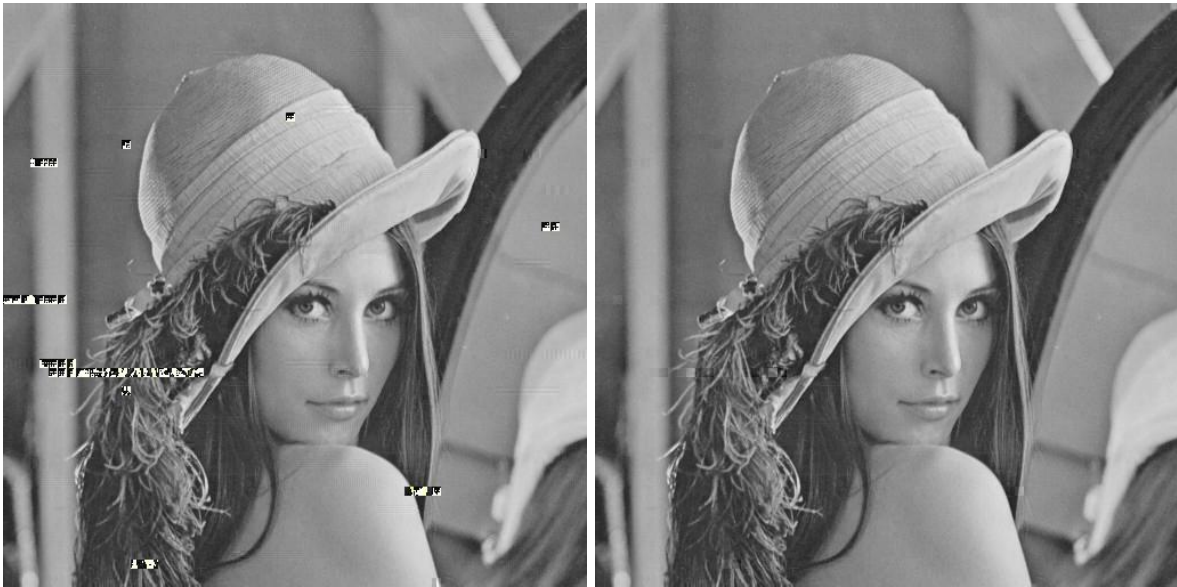
Figure 9. Result for the CCT transform ( \varepsilon = 0.02 ), without (left) and with (right) the global optimal estimator ( H = 5.35 \text{ bpp} ).
