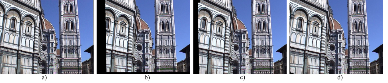
Fig. 4. Padding of pixels with additional frames: a) original left view of the sequence “Dome”, b) virtual right view, only rendered with the closest view of the camera path, c) virtual right view using 30 and d) 62 frames of the original sequence.
