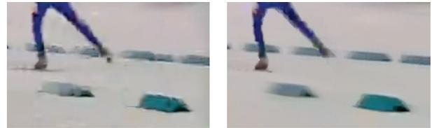
(a) H.264+In-loop deblocking filter, PSNR=28.63, R=53.71 kbits/s
