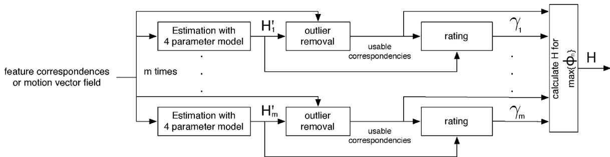
Fig. 5. Motion estimation on feature correspondences or motion vector fields based on the simplified HTE.
