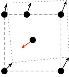
Fig. 1. Example of outlier rejection on motion vectors for PME. The dashed quadrangles represent the perspective deformation derived from the correct motion vectors. The vector in the middle does not belong to the model so it is declared as an outlier.
