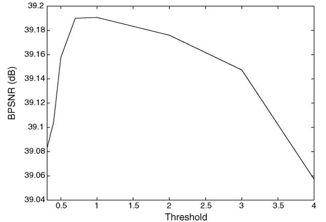
Fig. 8. BPSNR values for feature-based estimation with adaptive RANSAC on the *Biathlon* sequence with different error distance thresholds.
