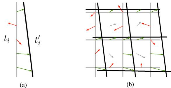
Fig. 4. Illustration of the two estimation steps proposed by Barcelo *et al.* for deriving perspective motion models. (a) Single line transformation. (b) PME from six line correspondences (gray vectors are not used).
