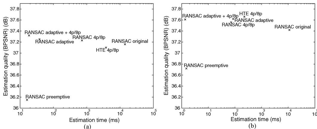
Fig. 10. Average estimation quality in terms of BPSNR (dB) over average estimation time (logarithmic) for the discussed PME methods (top left is better). (a) Estimation on H.264/AVC motion vector fields. (b) Estimation on KLT motion vector fields.
