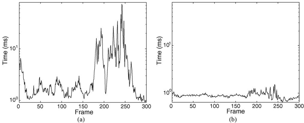
Fig. 9. Per frame runtime (logarithmic) comparison for adaptive RANSAC application on KLT feature vector fields for the *Stefan* sequence. (a) Without two-step simplification. (b) With two-step simplification.
