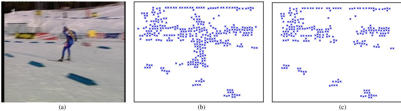
Fig. 3. Outlier rejection result for simplified HTE (with two-step scheme) for frame 30 of the *Biathlon* sequence. (a) Frame 30. (b) Selected features. (c) Filtered inliers.
