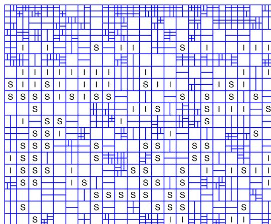
Fig. 7. Typical macroblock structure of a frame from the *Allstars CIF* sequence encoded with H.264/AVC. “I” blocks are of type intra, “S” blocks are of type skip, and empty blocks are of type inter and contain the motion vectors used for PME (motion vectors are omitted for clarity).
