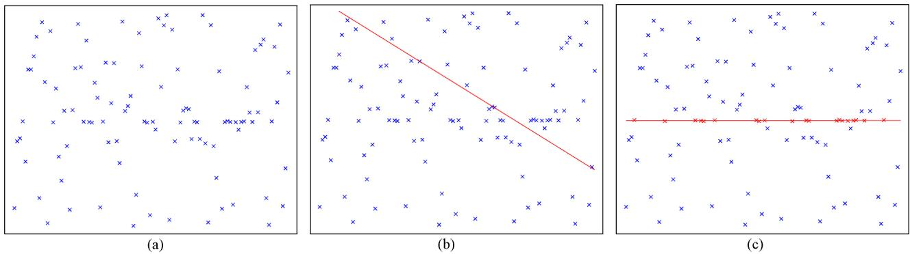
Fig. 2. Illustration of the robustness of the HTE: 20 noisy points of a line are placed between 80 outliers. (a) Original set. (b) Estimation result using LS. (c) Estimation result using HTE.
