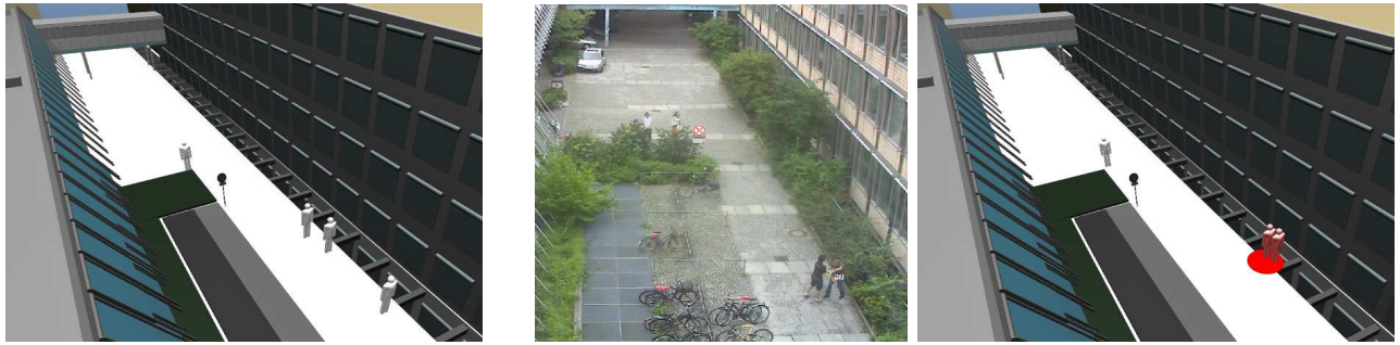
Fig. 8. Example of the GUI view for the mugging test sequence. From left to right: 3D model of our campus site with the pedestrian detections of the tracking module, video frame of mugging event with two involved persons and the detected mugging event with labeled pedestrian detections. It is visible that context information of the scenario is affected by the imperfect calibration.
