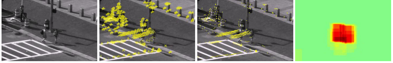
Fig. 1. Processing steps of estimating the proposed Multi-Person density. From left to right: Original video frame, extracted feature points and path lines influenced by camera shaking, stabilized path lines, color-coded Multi-Person density estimate.
