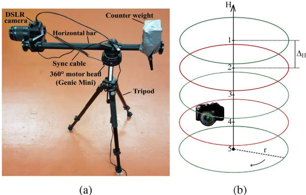
Figure 2: (a) Hardware setup and (b) Creation of vertical sub-aperture panorama images ( $r = 36.8\text{cm}$  and  $\Delta_H = 2.3\text{cm}$ ).
